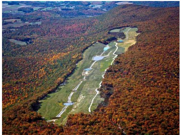
stone piles and 29 root wads with bole were placed throughout the nine wetlands created at the site. Near the end of the design phase, the property owner contacted BAMR about timbering the property prior to the start of construction. BAMR worked with the property owner to ensure that the timbering was completed before the start of the reclamation project.
