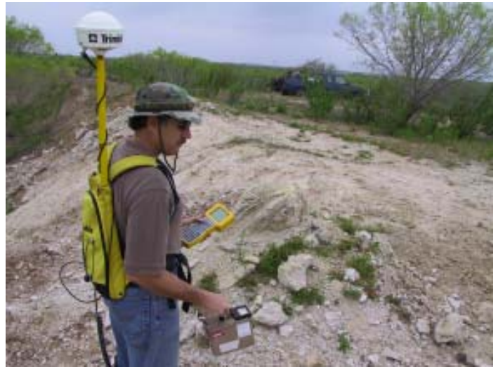
Bill Reimer, of the Texas AML staff, demonstrating use of ProXRS and scintillometer to conduct radiation surveys at the Brysch abandoned uranium site in south Texas. The TSC1 data collector, running Asset Surveyor software - detailed keypad allows easy data entry (both numbers and text) and background map shows selected features (fences, contour lines, etc.) and locations where data have been collected.
